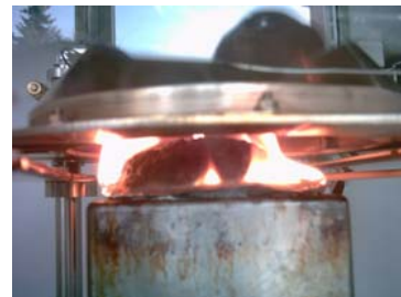
photo: cone calorimeter heater with specimen during measurement
